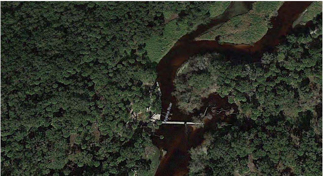
Aerial image showing river bypassing the structure of Downs' Dam where erosion is cutting into hydric hammock from MRSP.
